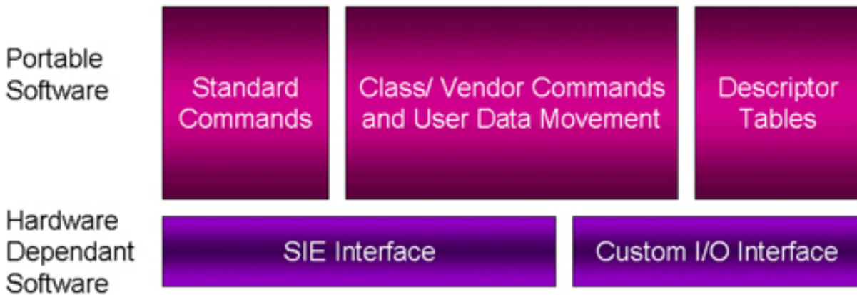
Figure 5 - I/O device software is partitioned
